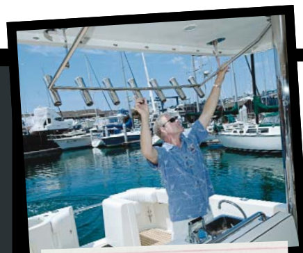
El Jefe's overhead rod racks are hinged to keep them out of the way but readily at hand.
