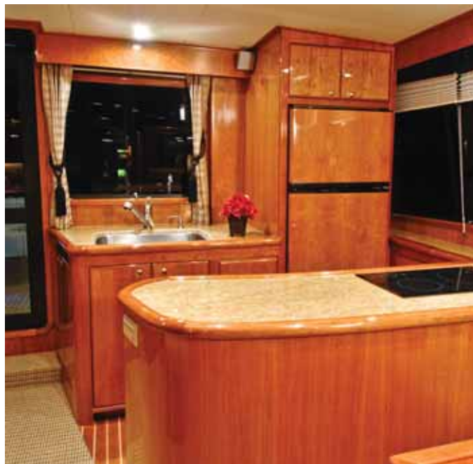
Locating the fridge forward against the bulkhead prevents food from falling out while underway.
