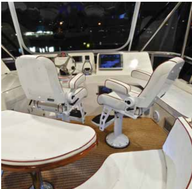
The flybridge combines an aft tournament station and forward helm with wrap-around electronics and control console.
